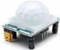
This motion sensor module uses the LHI778 Passive Infrared Sensor and the BISS0001 IC to control how motion is detected.
